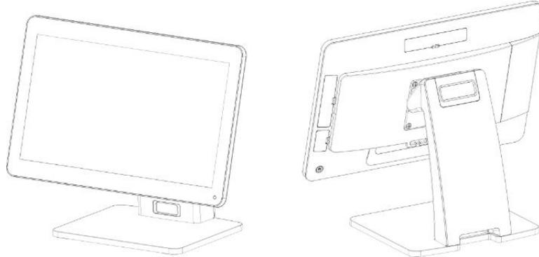
Single-screen Device, length \* width \* height: 405 \* 210 \* 330; main screen flip range: 0-45 degrees
