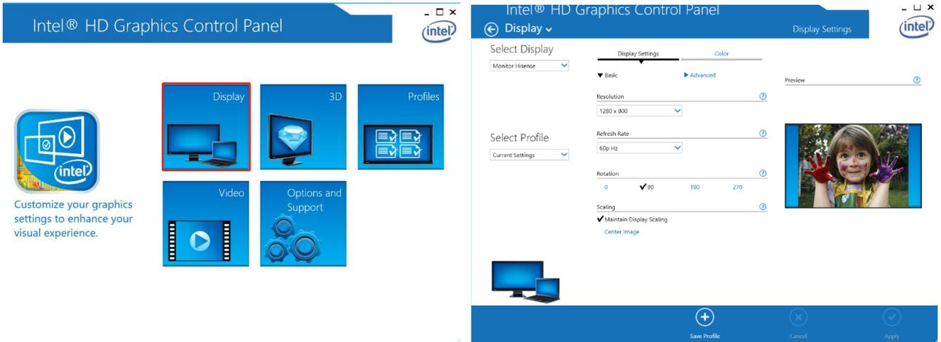
Monitor Hisense is selected in blank 1, resolution can be adjusted in blank 2, rotation direction of secondary screen can be adjusted in blank 3, and setting can be saved in blank 4.
