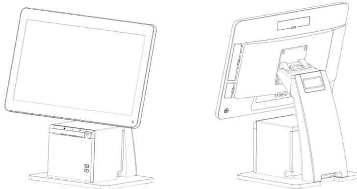
Screen High position + printer, length \* width \* height: 405 \* 250 \* 420
