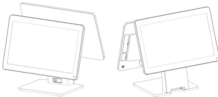
Dual-screen Device, length \* width \* height: 405 \* 250 \* 370; main screen flip range: 0-45 and second screen flip angle 0-30.
